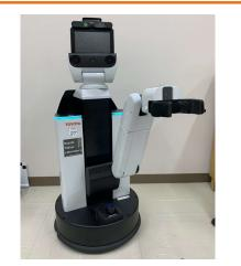
We have developed a restroom cleaning system that can be used for a general home as well as a convenience store. This system has a mobile manipulator, and the robot can use a common cleaning tool to wipe the toilet bowl. This system works even if the position of the trash can and mop changes because of the object recognition technology.
