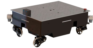
Active caster type omnidirectional mobile
