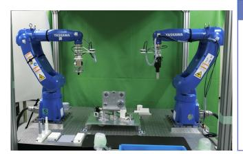
Accurate motion is performed by using vison sensor and force sensor. We have developed sensing modules for high success rate. For examples, the screw position is measured by vision sensor accurately. The contact force is measured by force sensor and controlled.
