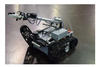
Pariprekshya is a teleoperated light weight UGV (Unmanned Ground Vehicle) robot, capable of doing complex maneuvering, mobility and dexterity tasks for search and rescue operations.
