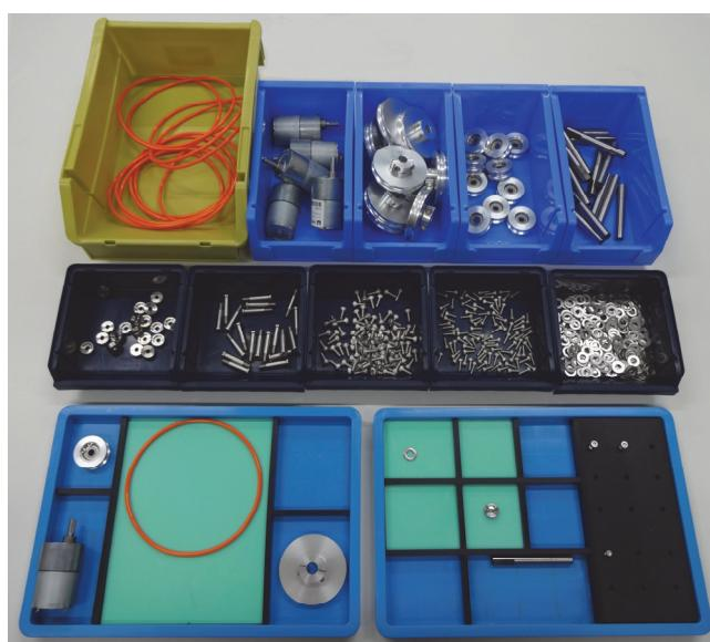
Figure 11: Conceptual Drawing of the Overall Layout of the Kitting Task and a Snapshot of the Actual Parts, Parts Bins, and Part-kitting Trays.
