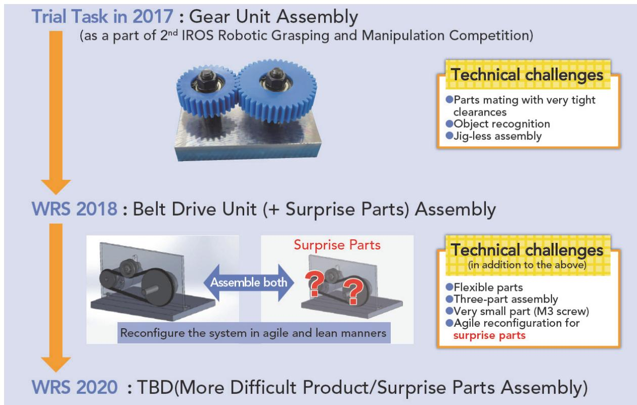
Figure 2: Transition of the Competition Tasks and the Technical Challenges from the 2017 Trial Task to the WRS 2020 in the Industrial Robotics Category
